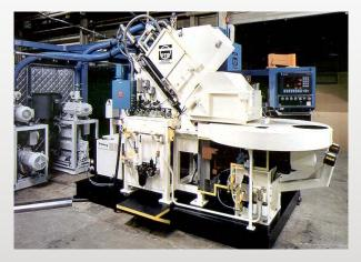
Small chamber welder suitable for use in aircraft, sensor, medical, semiconductor and other industries for joining a variety of parts and materials.
