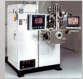
Large chamber welder simultaneously utilizing up to 9 CNC axes of beam parameter and part motion control for the most demanding welding tasks.
